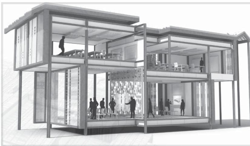
David Fleming from the University of Cincinnati won the award for the student-designed building with his “[Un] Modular Design for Deconstruction” shown here. His adaptable structural system can change almost any element of the building, and shows the potential for a building that can evolve with time and innovations in materials and styles change.
